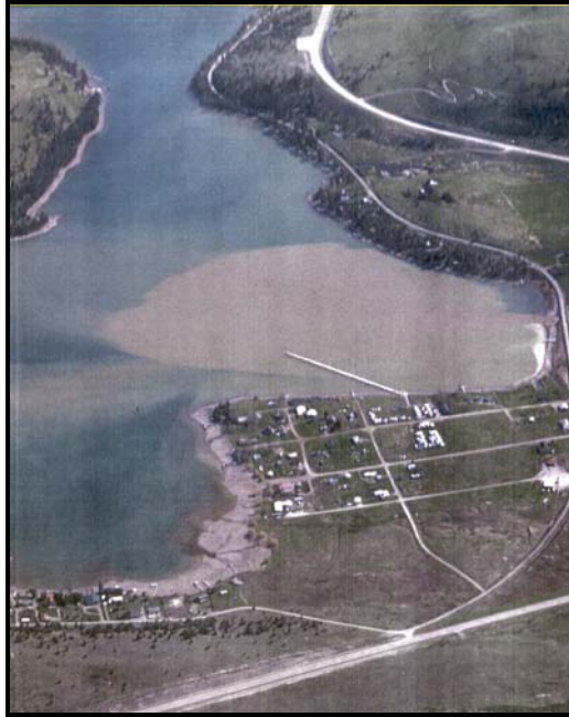
Figure 16. Sediment plume in Flathead Lake resulting from road-crossing failures in the Dayton Creek watershed.
