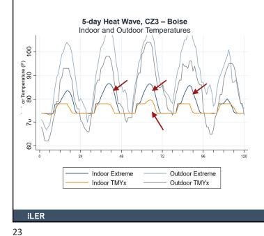
Typical Boise heat wave already stresses 4-ton AC – thermostat temperature slightly exceeded for a few hours on third day.
