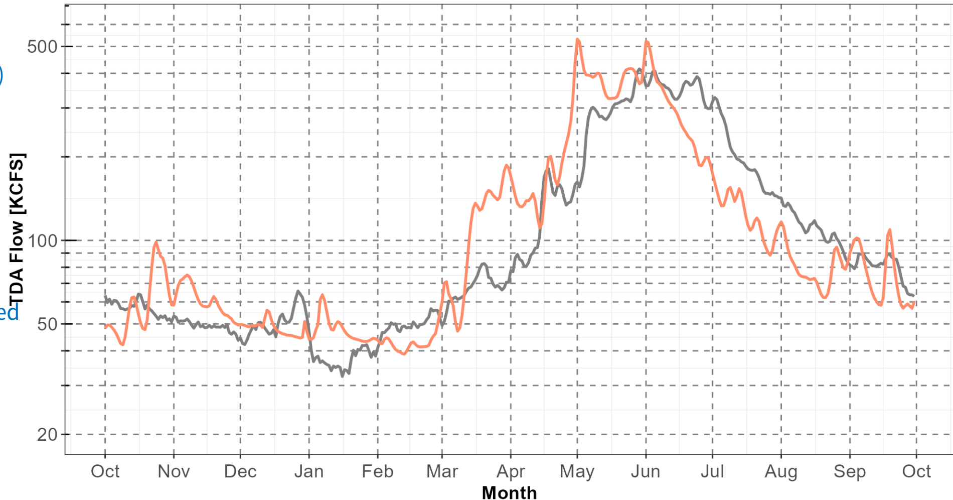
TDA Modified Flow Traces for Historical 1937 Water Year and CanESM2 2025 Water Year
