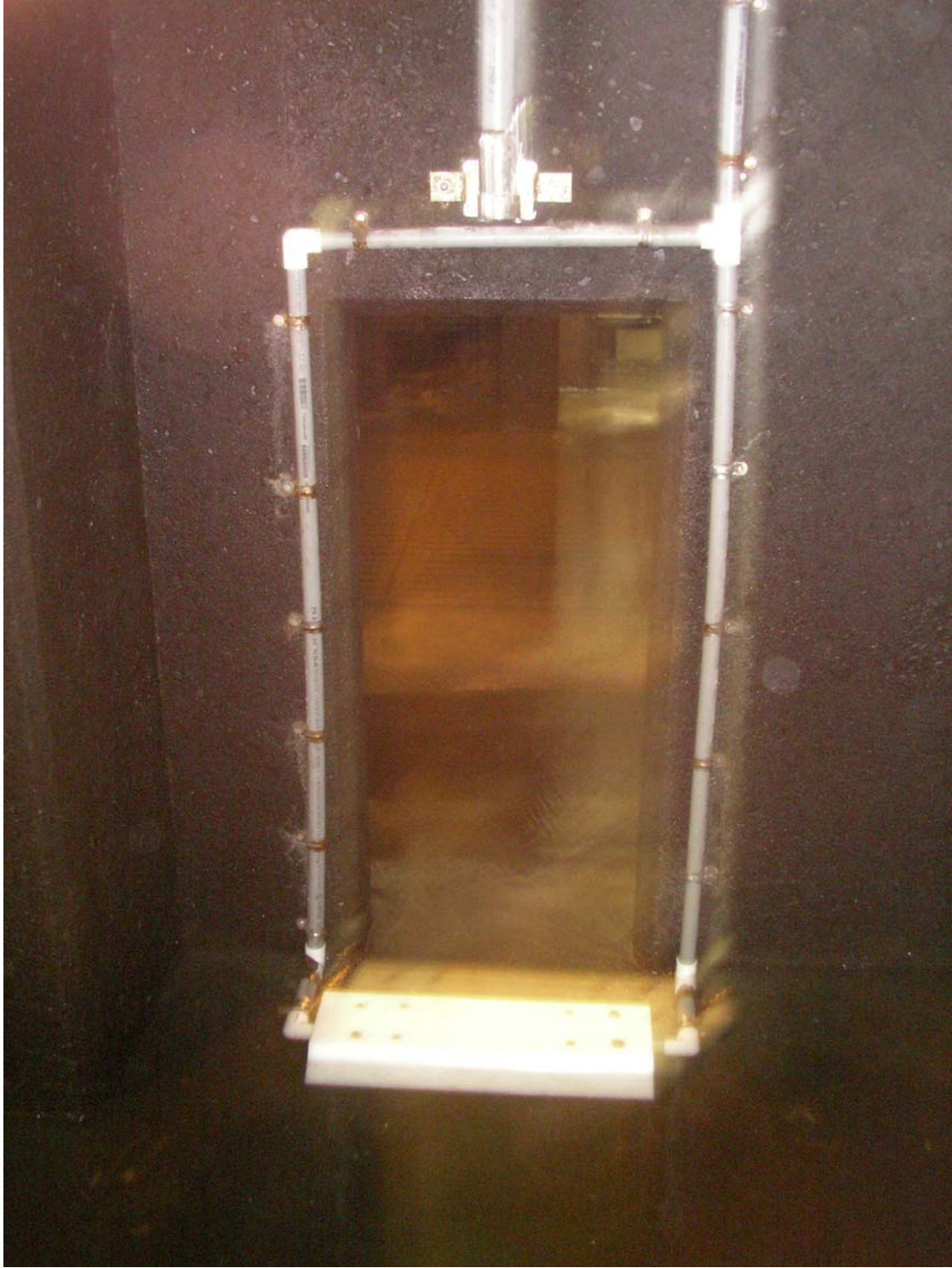
Figure 4. HDX loop antenna and camera installed in Willamette Falls fish ladder ( second site ), Willamette River, November 2010.
