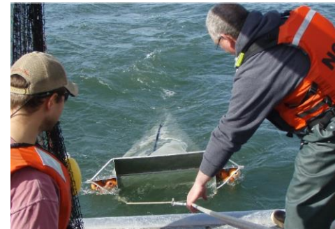
Neuston (surface plankton net)
