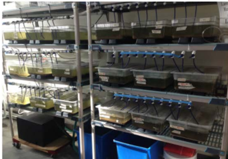
Figure 5-12. Recirculating water trough (left) and tank rack (right) with interchangeable Cambro
