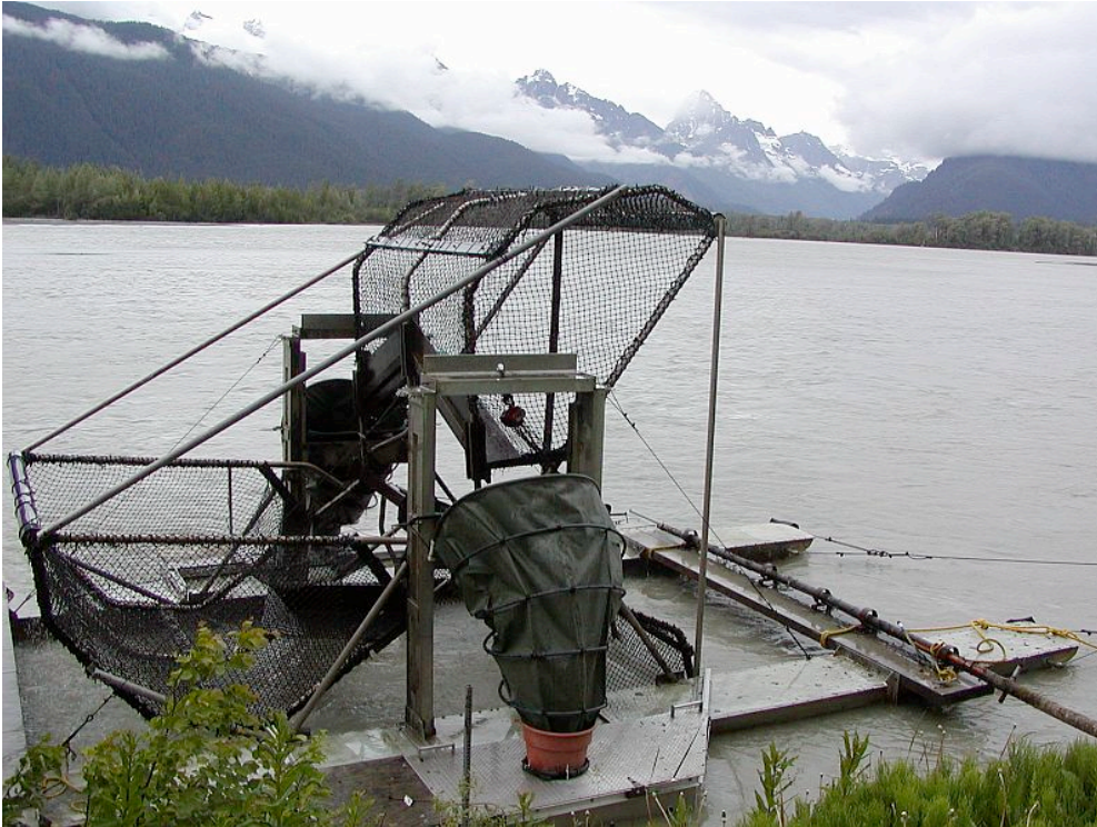
Figure 15. Two-basket aluminum fish wheel ( home.att.net ).
