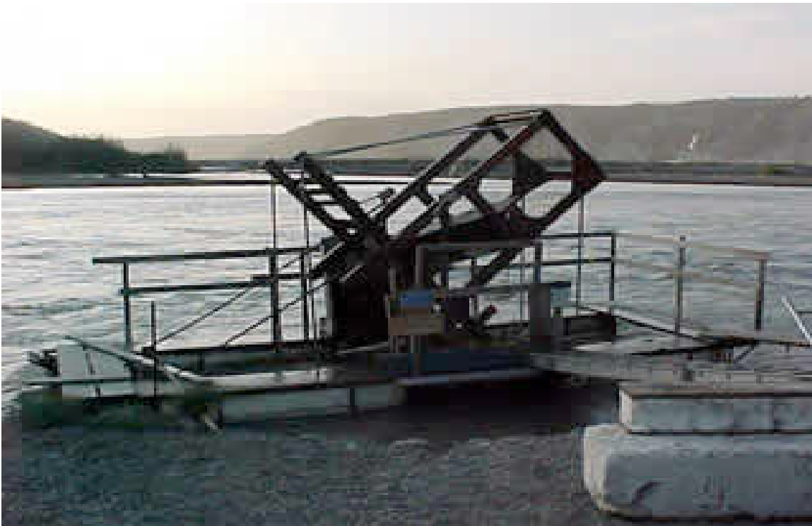
Figure 14. Two-basket fish wheel constructed of wood and styrofoam panels ( taleblazing.com ).
