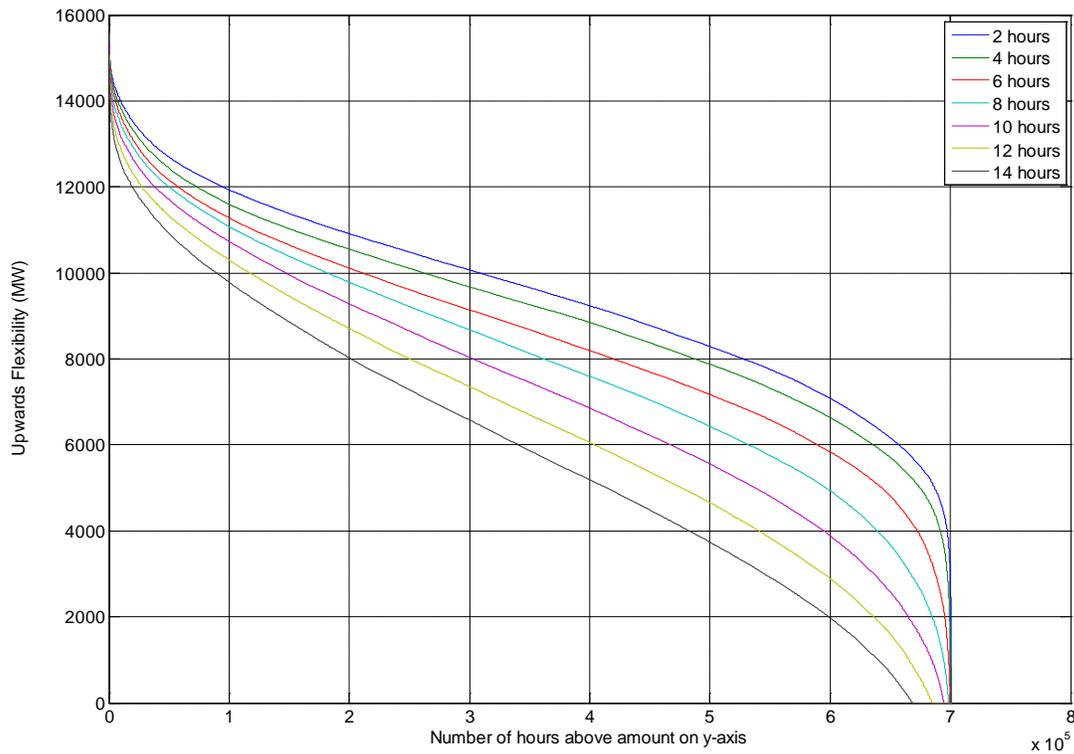
**Figure 9: Available upwards flexibility form hydro for different time horizons based on 80 years of hourly data**
