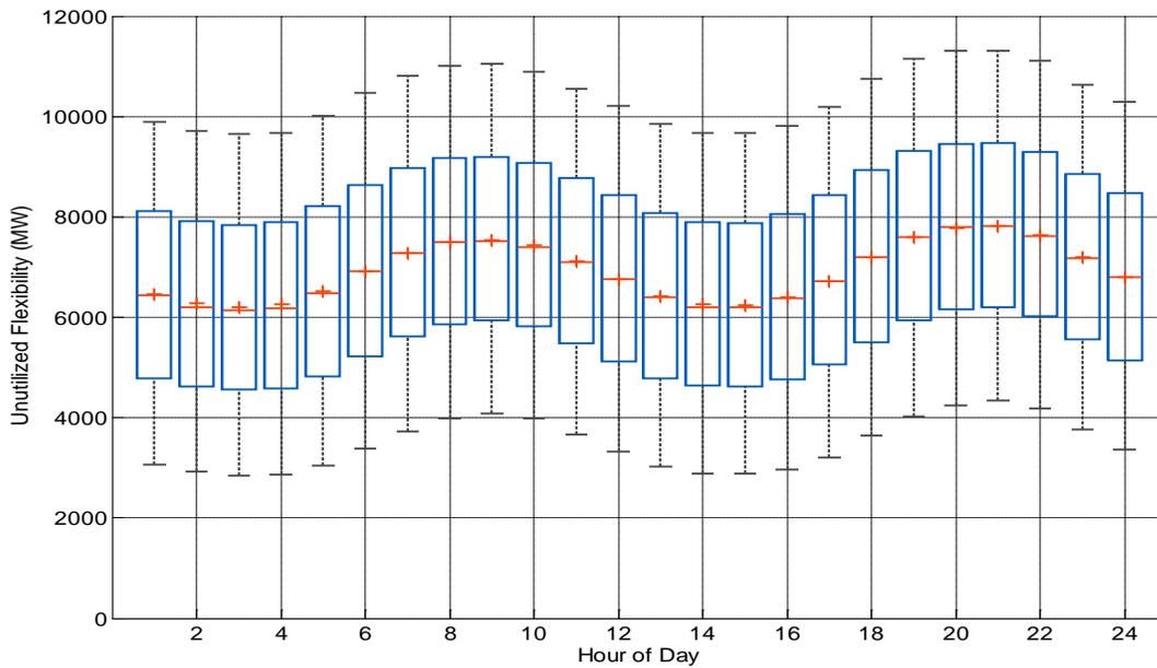
Figure 51: Box plots showing mean (line), median (cross), 25<sup>th</sup>/75<sup>th</sup> percentiles (box) and 9<sup>th</sup>/91<sup>st</sup> percentiles (whiskers) for unutilized 2 hour downwards ramping capability on an hourly basis
