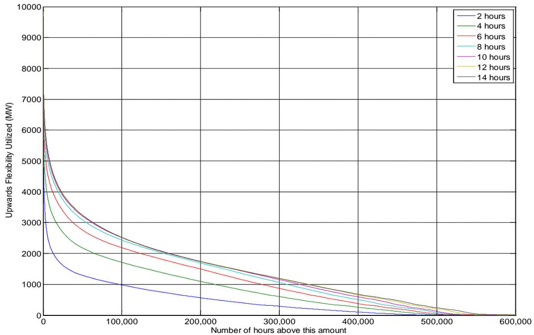
**Figure 27: Duration Curves of Downwards Ramping Actually Deployed on Thermal and Hydro Generation based on 80 years of hourly data**
