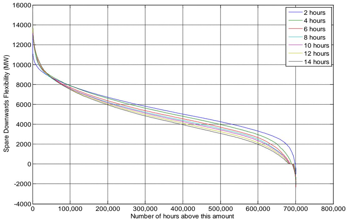
**Figure 37: Duration Curves for Spare Downwards Flexibility when utilized hydro flexibility is subtracted from available hydro flexibility, for hydro generation over 80 years of hourly data**
