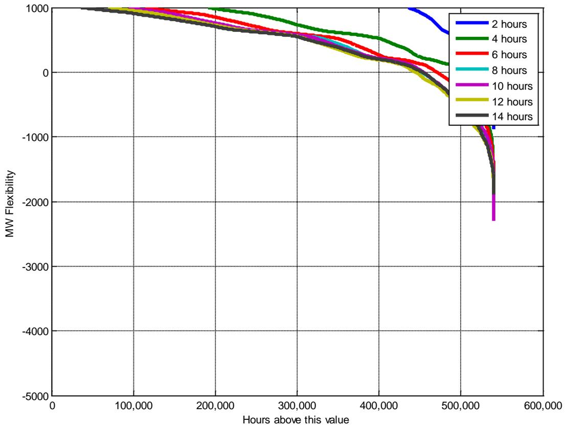
Figure 46: Figure 47: Unutilized upwards flexibility for different time horizons less than 1,000MW
