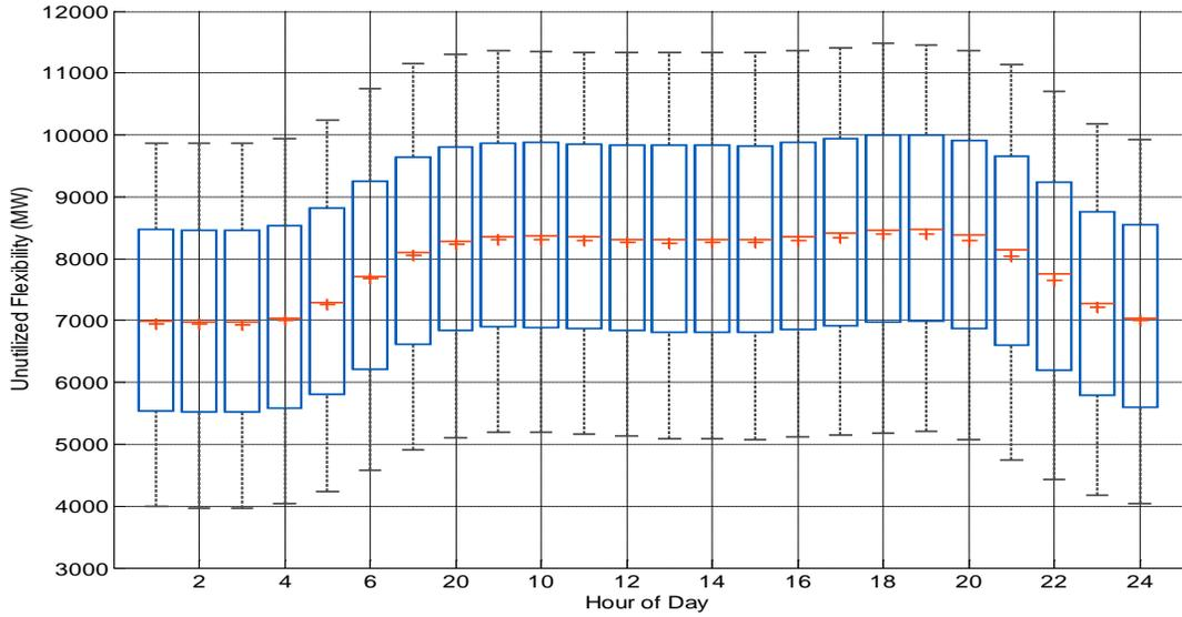
Figure 50: Box plots showing mean (line), median (cross), 25th/75<sup>th</sup> percentiles (box) and 9<sup>th</sup>/91<sup>st</sup> percentiles (whiskers) for unutilized 2 hour downwards ramping capability on an hourly basis
