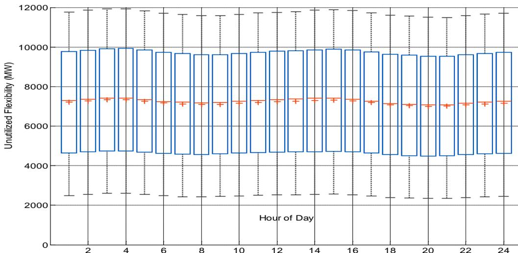
Figure 44: Box plots showing mean (line), median (cross), 25th/75<sup>th</sup> percentiles (box) and 9<sup>th</sup>/91<sup>st</sup> percentiles (whiskers) for unutilized 12 hour upwards ramping capability on an hourly basis
