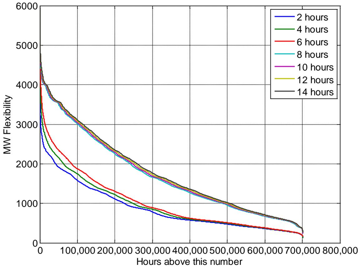
Figure 7: Duration curve of upwards flexibility from thermal generation based on 80 years of hourly data
