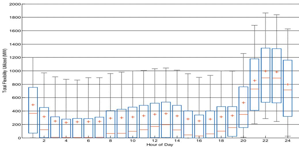
Figure 32: Box plots showing mean (line), median (cross), 25th/75<sup>th</sup> percentiles (box) and 9<sup>th</sup>/91<sup>st</sup> percentiles (whiskers) for 2 hour downwards ramping deployed by hour
