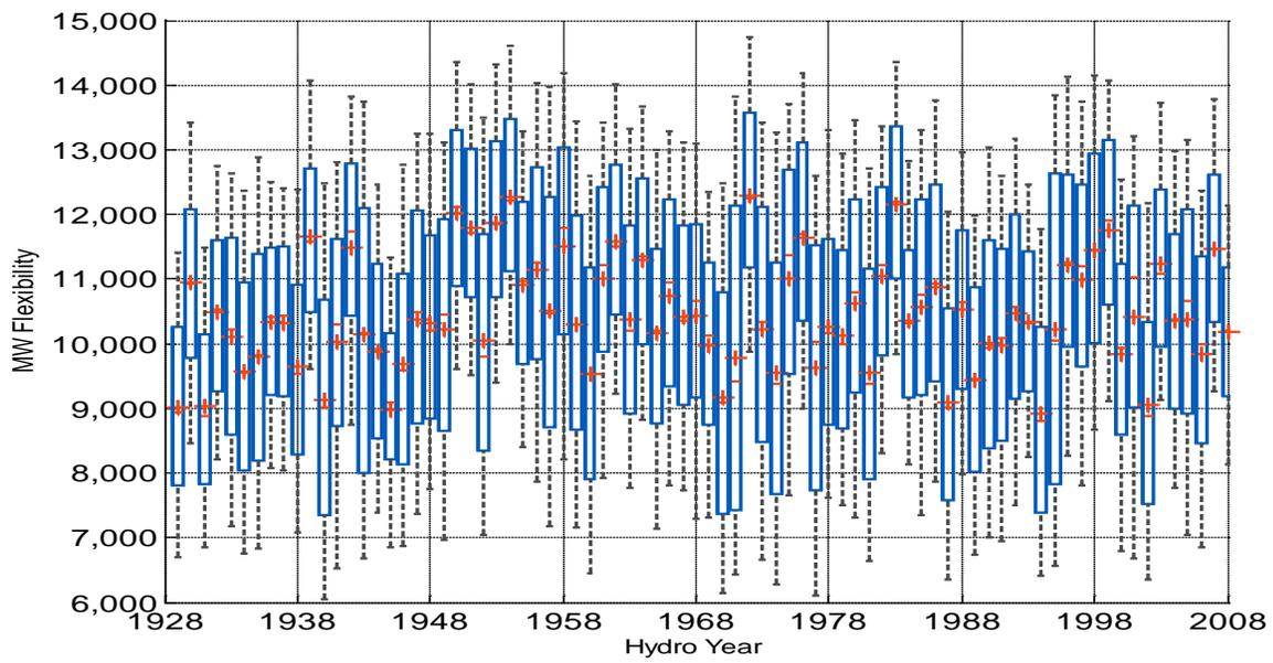
Figure 20: Two hour available upwards flexibility by year of analysis
