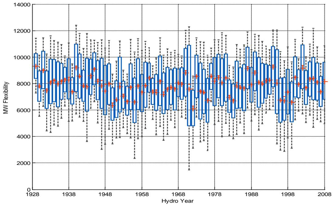
Figure 53: Box plots showing mean (line), median (cross), 25th/75<sup>th</sup> percentiles (box) and 9<sup>th</sup>/91<sup>st</sup> percentiles (whiskers) for unutilized downwards flexibility when considering both hydro and thermal generation by hydro year
