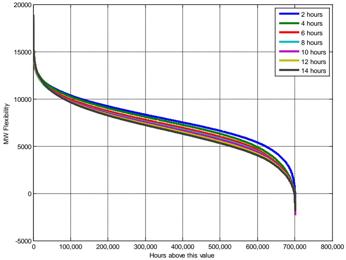
Figure 45: Duration Curves for Spare Downwards Flexibility when utilized hydro and thermal flexibility is subtracted from available hydro and thermal flexibility, based on 80 years of hourly data
