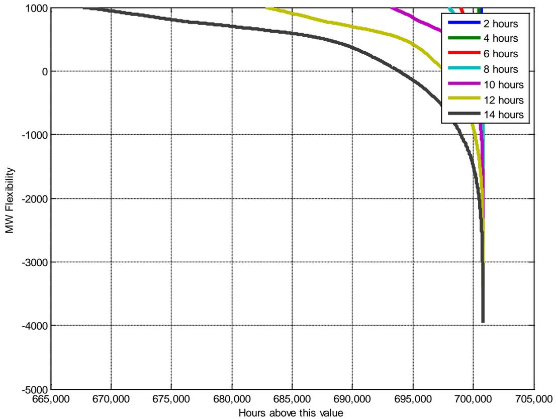
**Figure 40: Unused upwards flexibility for different time horizons less than 1,000MW**
