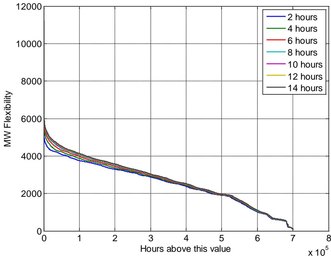
Figure 8: Duration Curve for downwards flexibility for thermal generation based on 80 years of hourly data
