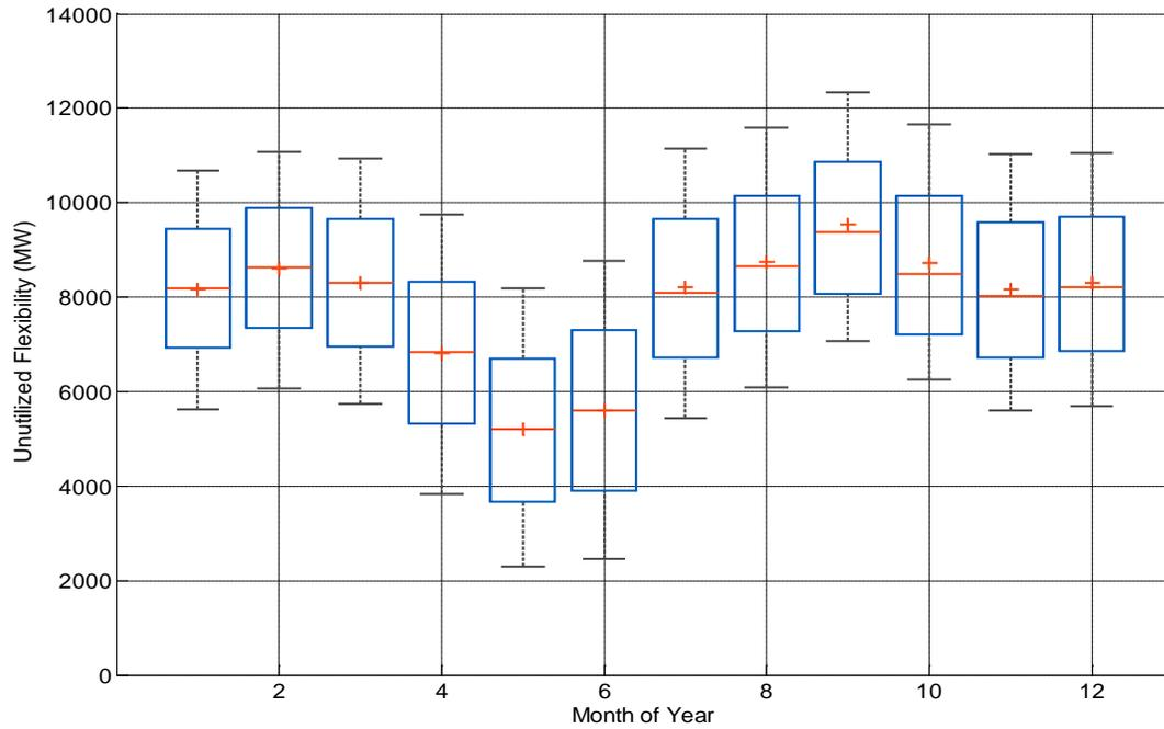
Figure 48: Box plots showing mean (line), median (cross), 25th/75<sup>th</sup> percentiles (box) and 9<sup>th</sup>/91<sup>st</sup> percentiles (whiskers) for unutilized 2 hour downwards ramping capability on a monthly basis
