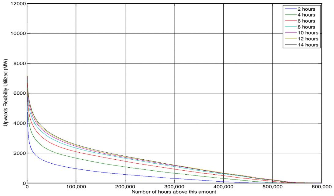
Figure 26: Duration Curves of Upwards Ramping Actually Deployed on Thermal and Hydro Generation based on 80 years of hourly data
