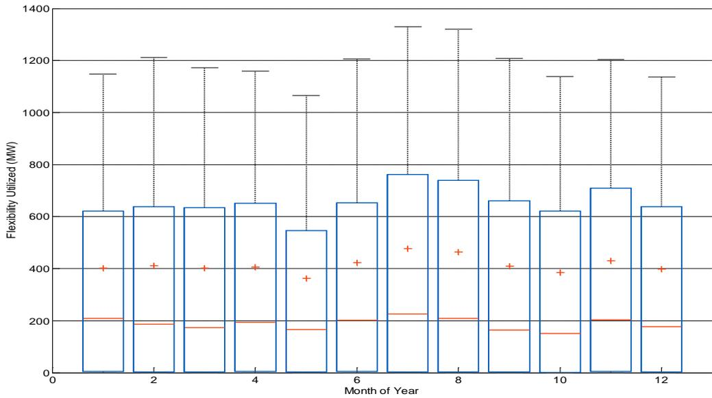
Figure 29: Box plots showing mean (line), median (cross), 25th/75<sup>th</sup> percentiles (box) and 9<sup>th</sup>/91<sup>st</sup> percentiles (whiskers) for 2 hour downwards ramping deployed by month
