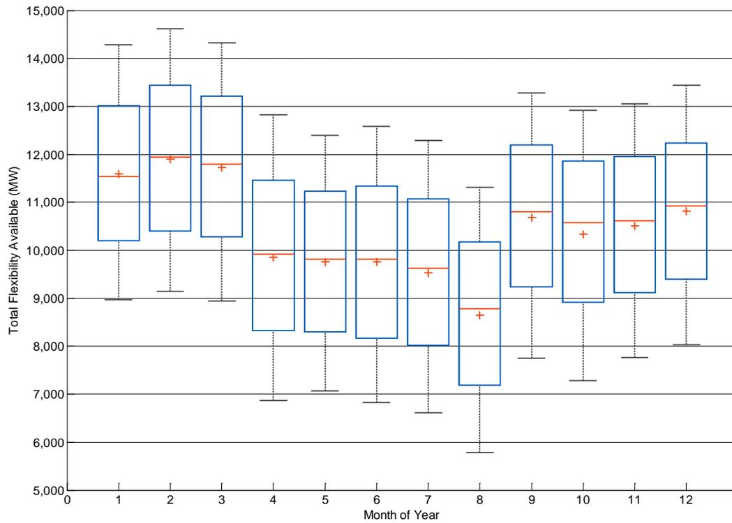
Figure 13: Box Plots for available upwards 2 hour flexibility by month. The box shows the 25th to 75th percentile of data, the whiskers show 9th to 91st percentiles, the line shows mean and the cross shows the median
