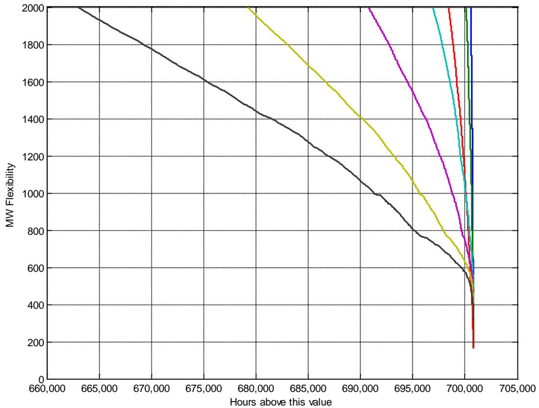
**Figure 12: Total Upwards Flexibility for different time horizons, for periods with less than 2000 MW available**
