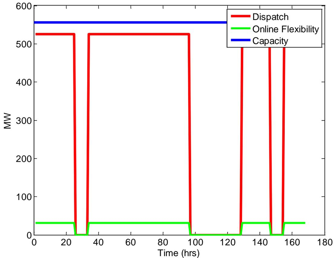
Figure 3: Generator Dispatch, Installed Capacity and Upwards Flexibility Available from online generation
