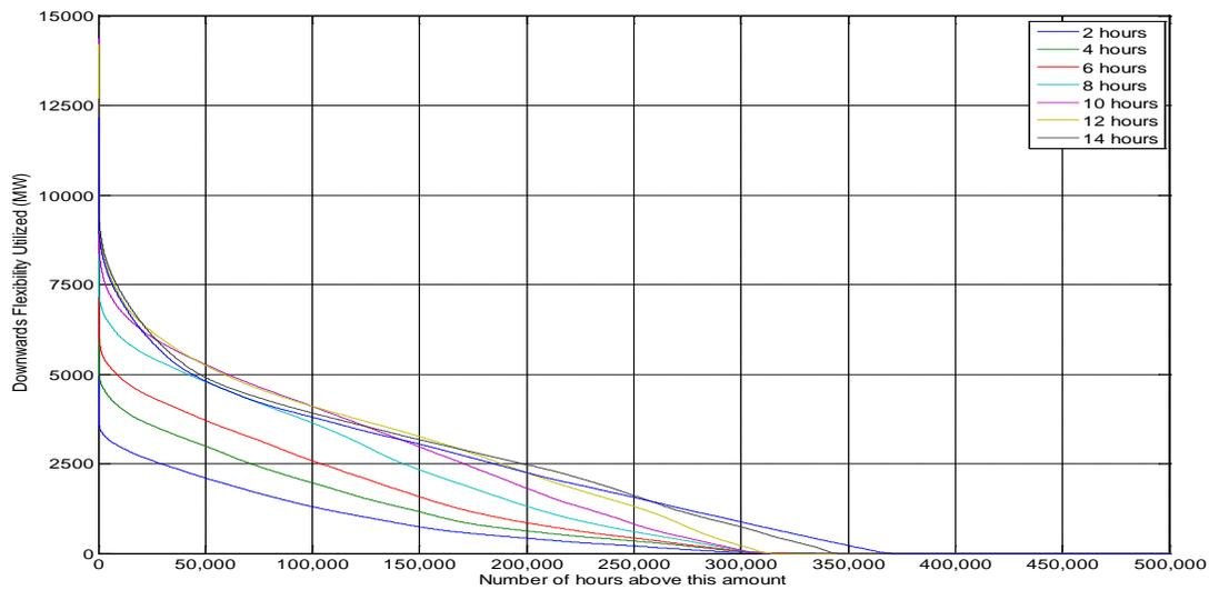
Figure 25: Duration Curves of Downwards Ramping Actually Deployed on Hydro Generation based on 80 years of hourly data
