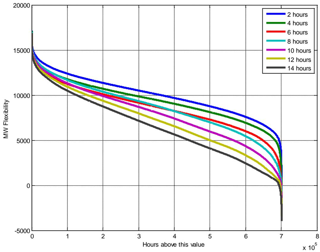
Figure 39: Duration Curves for Spare Upwards Flexibility when utilized hydro and thermal flexibility is subtracted from available hydro and thermal flexibility, based on 80 years of hourly data
