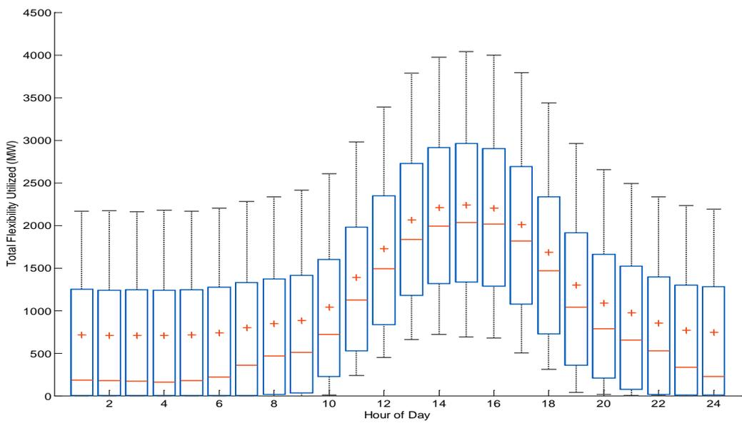
Figure 33: Box plots showing mean (line), median (cross), 25th/75<sup>th</sup> percentiles (box) and 9<sup>th</sup>/91<sup>st</sup> percentiles (whiskers) for 10 hour downwards ramping deployed by hour
