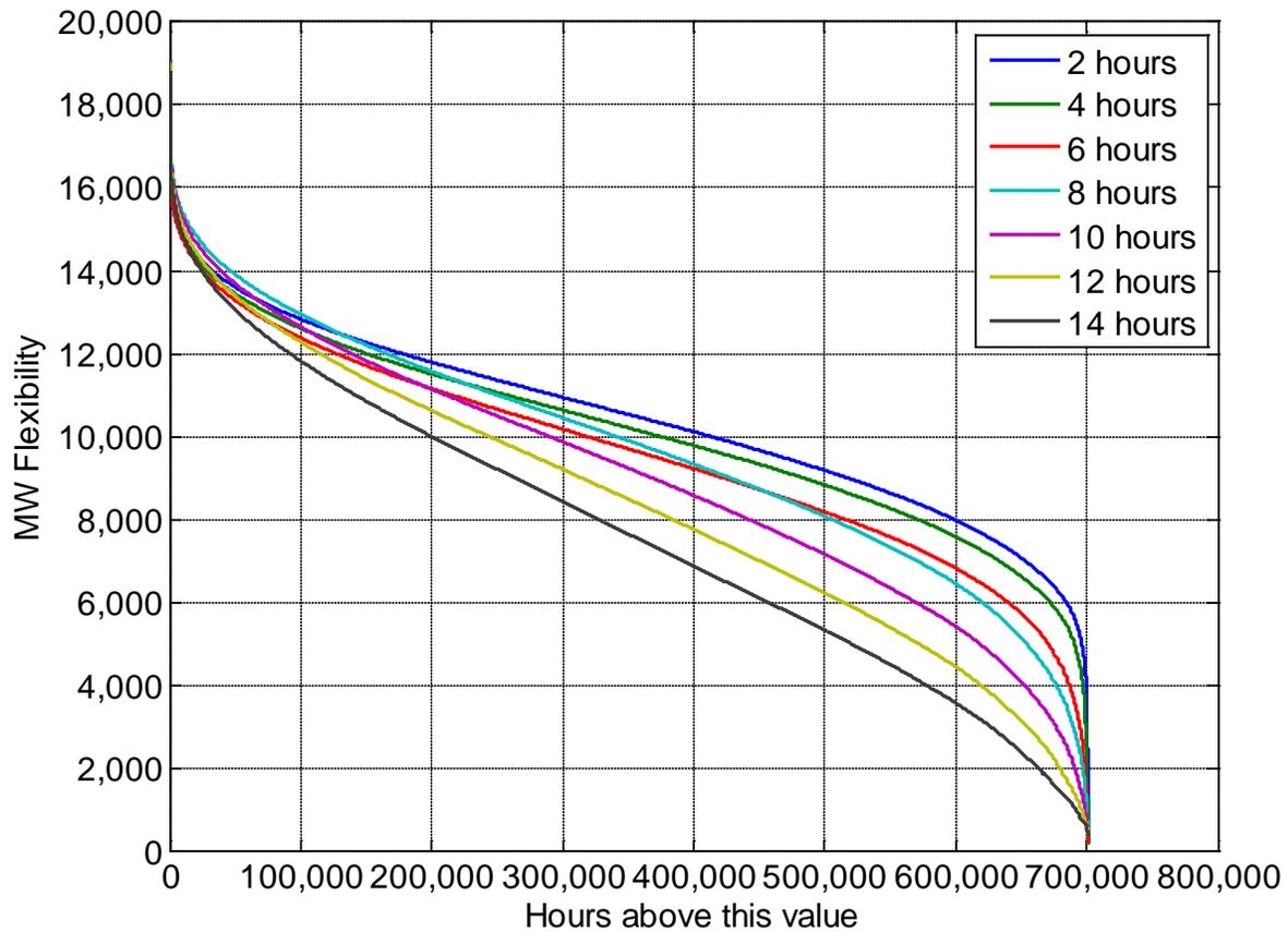
Figure 11: Total Upwards Flexibility available from thermal and hydro for different time horizons based on 80 years of data
