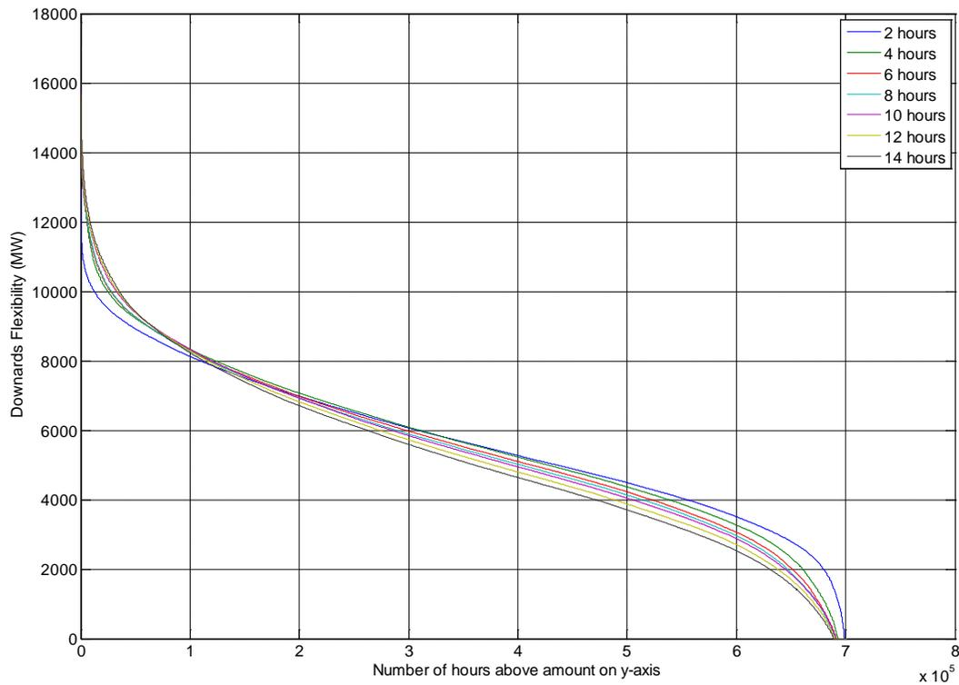
**Figure 10: Downwards flexibility from hydro for different time horizons based on 80 years of hourly data**
