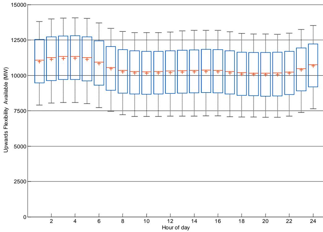
Figure 15: Box plots of 2 hour upwards available flexibility by time of day
