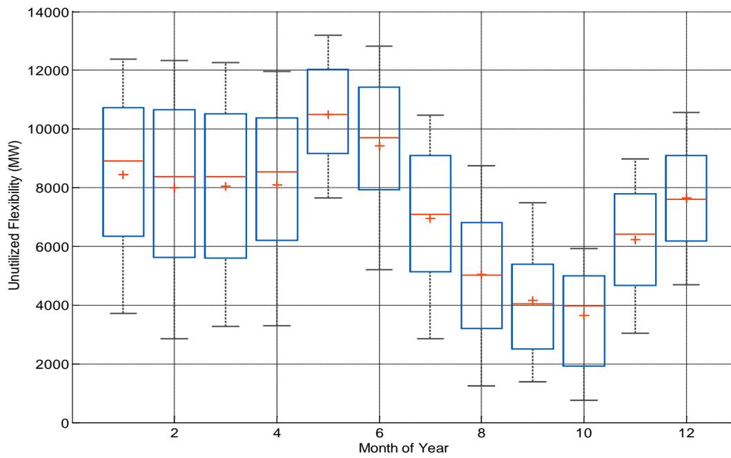
Figure 42: Box plots showing mean (line), median (cross), 25th/75<sup>th</sup> percentiles (box) and 9<sup>th</sup>/91<sup>st</sup> percentiles (whiskers) for unutilized 12 hour upwards ramping capability on a monthly basis
