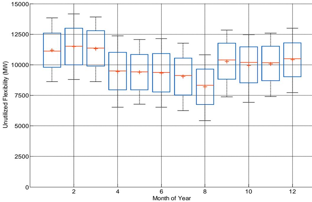
Figure 41: Box plots showing mean (line), median (cross), 25th/75<sup>th</sup> percentiles (box) and 9<sup>th</sup>/91<sup>st</sup> percentiles (whiskers) for unutilized 2 hour upwards ramping capability on a monthly basis
