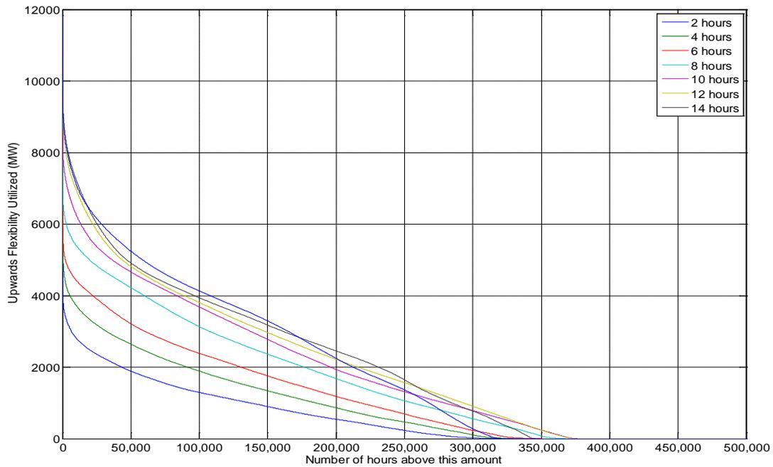
Figure 24: Duration Curves of Upwards Ramping Actually Deployed on Hydro Generation based on 80 years of hourly data
