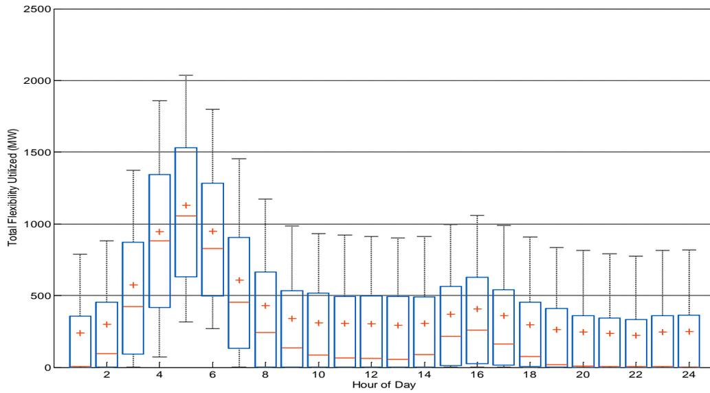
Figure 30: Box plots showing mean (line), median (cross), 25th/75<sup>th</sup> percentiles (box) and 9<sup>th</sup>/91<sup>st</sup> percentiles (whiskers) for 2 hour upwards ramping deployed by hour
