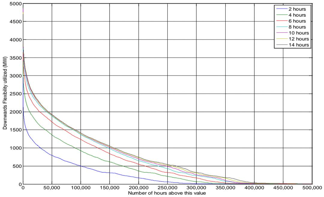
**Figure 23: Duration Curves of Downwards Ramping Actually Deployed on Thermal Generation based on 80 years of hourly data**
