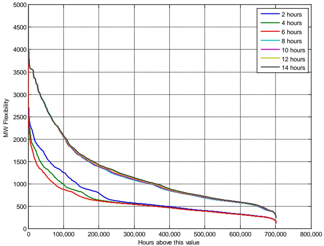
**Figure 34: Duration Curves for Spare Upwards Flexibility on thermal generation when Utilized Flexibility is subtracted from Available, over 80 years of hourly data**
