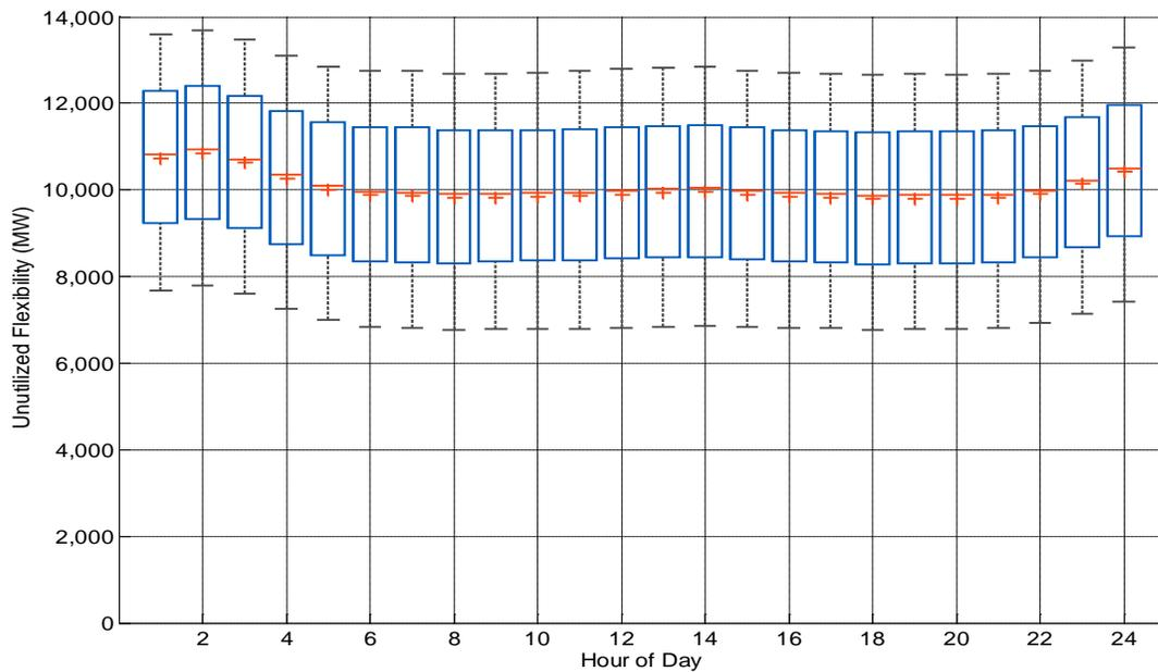
Figure 43: Box plots showing mean (line), median (cross), 25th/75<sup>th</sup> percentiles (box) and 9<sup>th</sup>/91<sup>st</sup> percentiles (whiskers) for unutilized 2 hour upwards ramping capability on an hourly basis
