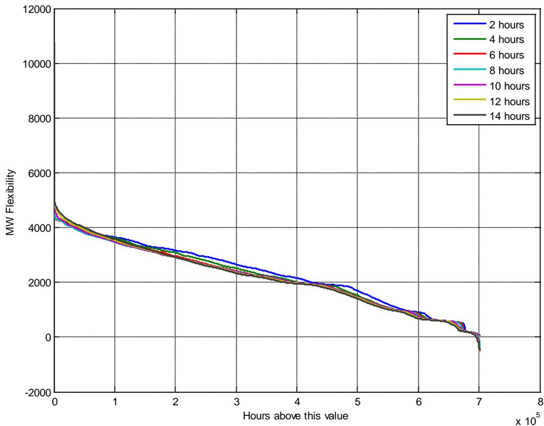
**Figure 35: Duration Curves for Spare Downwards Flexibility on thermal generation when utilized flexibility is subtracted from available flexibility, for thermal generation over 80 years of hourly data**
