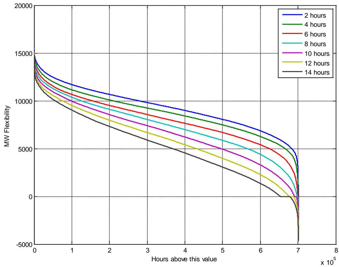
Figure 36: Duration Curves for Spare Upwards Flexibility when utilized hydro flexibility is subtracted from available hydro flexibility, for hydro generation over 80 years of hourly data
