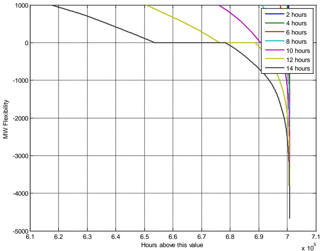
**Figure 38: Spare hydro upwards flexibility capability for those periods less than 1000 MW available after accounting for flexibility used**
