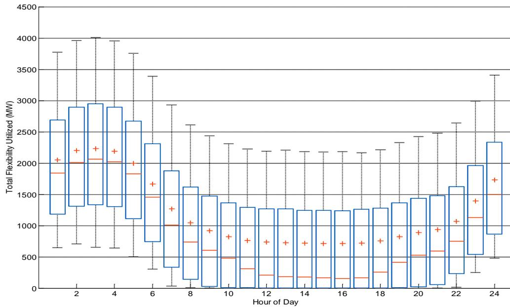
Figure 31: Box plots showing mean (line), median (cross), 25th/75<sup>th</sup> percentiles (box) and 9<sup>th</sup>/91<sup>st</sup> percentiles (whiskers) for 12 hour upwards ramping deployed by hour
