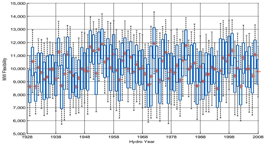
Figure 52: Box plots showing mean (line), median (cross), 25th/75<sup>th</sup> percentiles (box) and 9<sup>th</sup>/91<sup>st</sup> percentiles (whiskers) for unutilized upwards flexibility when considering both hydro and thermal generation by hydro year
