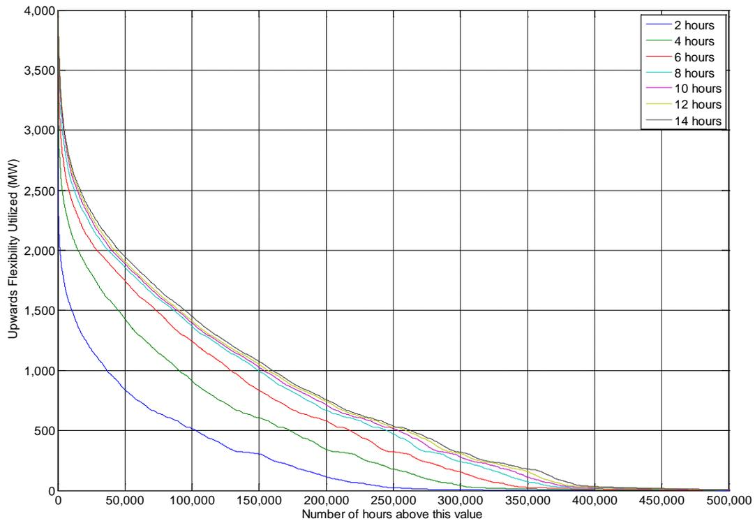
Figure 22: Duration Curves of Upwards Ramping Actually Deployed on Thermal Generation based on 80 years of hourly data
