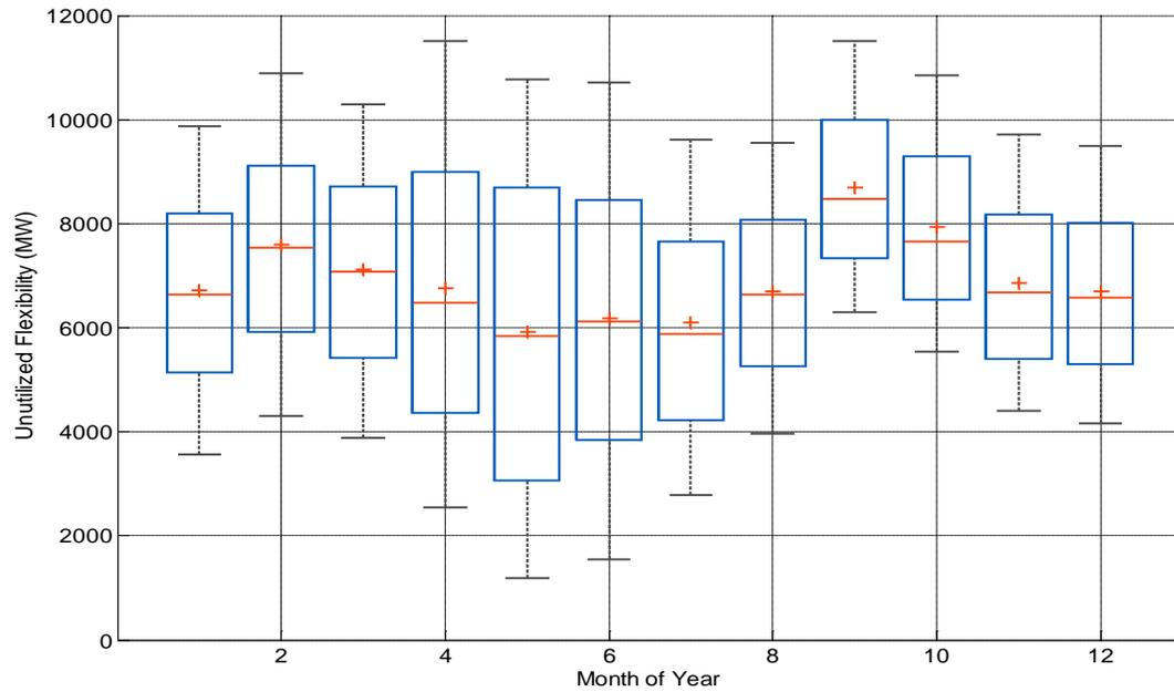
Figure 49: Box plots showing mean (line), median (cross), 25th/75<sup>th</sup> percentiles (box) and 9<sup>th</sup>/91<sup>st</sup> percentiles (whiskers) for unutilized 12 hour downwards ramping capability on a monthly basis
