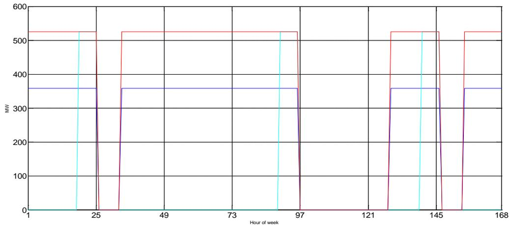
**Figure 5: Downwards Flexibility Capability of example thermal plant**
