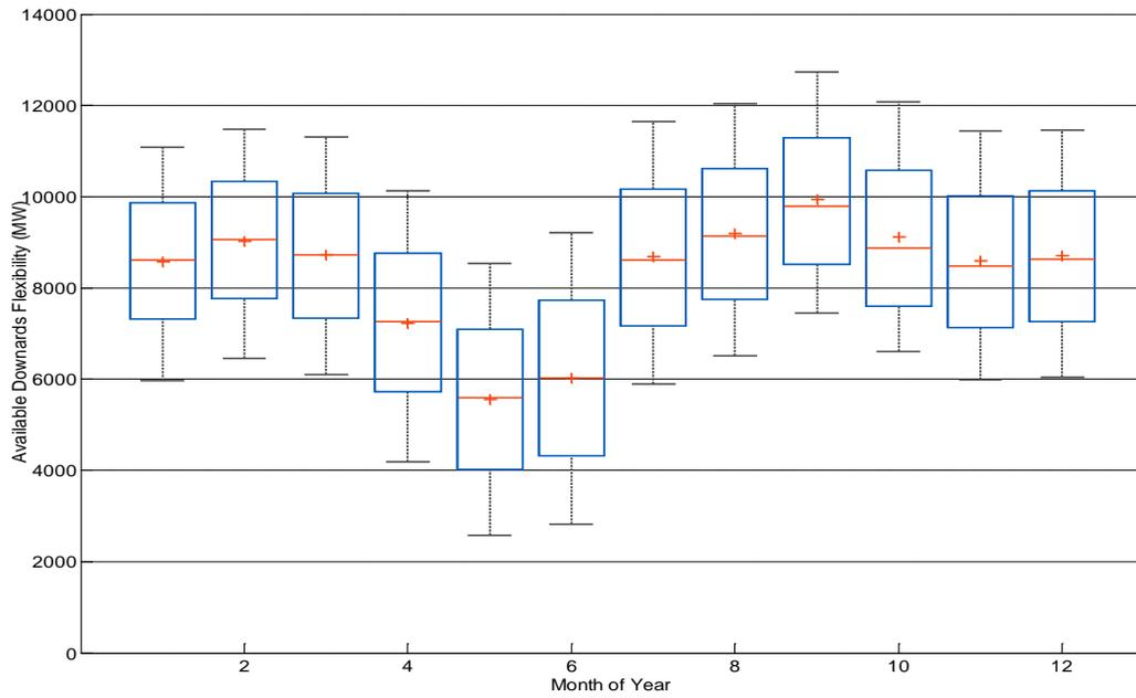
Figure 17: Box plots showing Monthly Available 2 hour downwards flexibility based on 80 years of data
